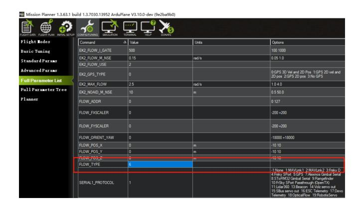
4. After setting the parameters, click "Write Params". Go to the "Actions" tag in "flight Data" page. Select "PREFLIGHT\_REBOOT\_SHUTDOW" then click "Do Action" to reboot the flight controller.
